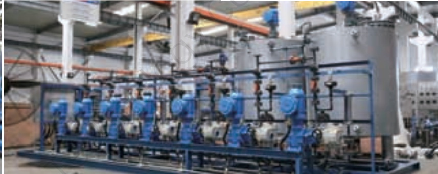
Sulfuric Acid (H 2 SO 4 ), Sodium Hypochlorite (NaClO) and Stabilizer Injection System
